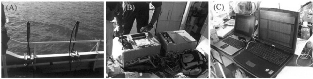
Fig. 9 Scenes of the field experiment by the research vessel “Hokuto”. (A) Sound source and hydrophone mounted on the ship’s side. (B) The SBP SH-20. (C) Digital recording by the SBP digitizer.
