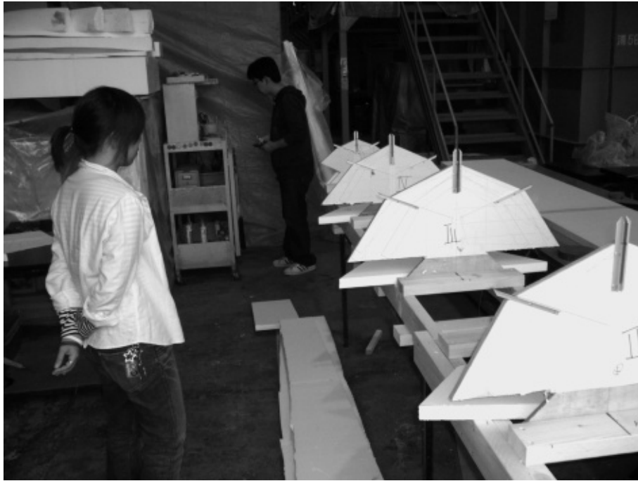
Photo 4 A block with hull sections and cutting guide.
