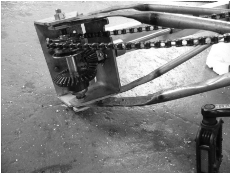
Photo 2 Bevel gear connected with sprocket and bicycle frame.
