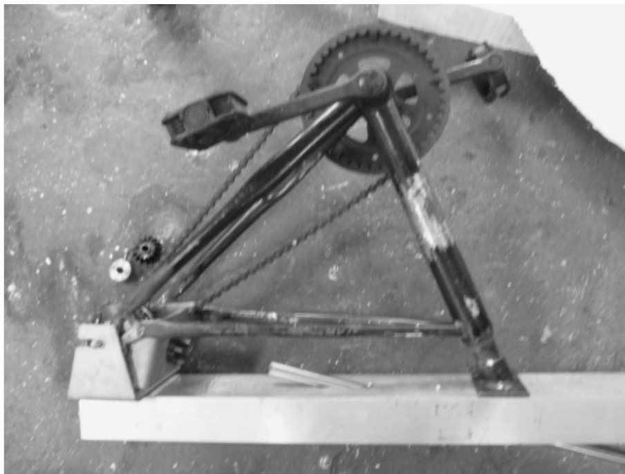
Photo 3 Newly designed pedal drive system. Left is set to the bow side.
