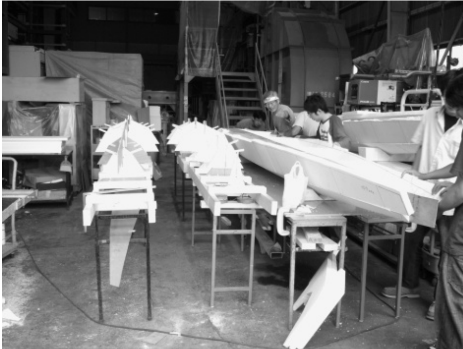
Photo 13 The hull removed from a block after the bottom plate connection.
