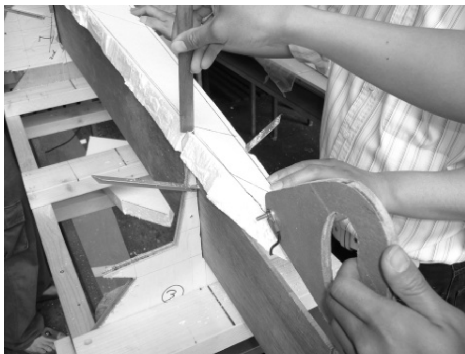
Photo 8 Cutting process using the hot wire.
