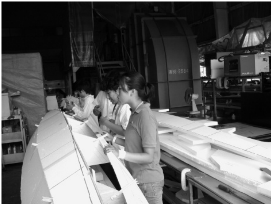
Photo 10 Setting of the light bottom panel. If the cutting surface is accurate, fair hull form is easily built up.
