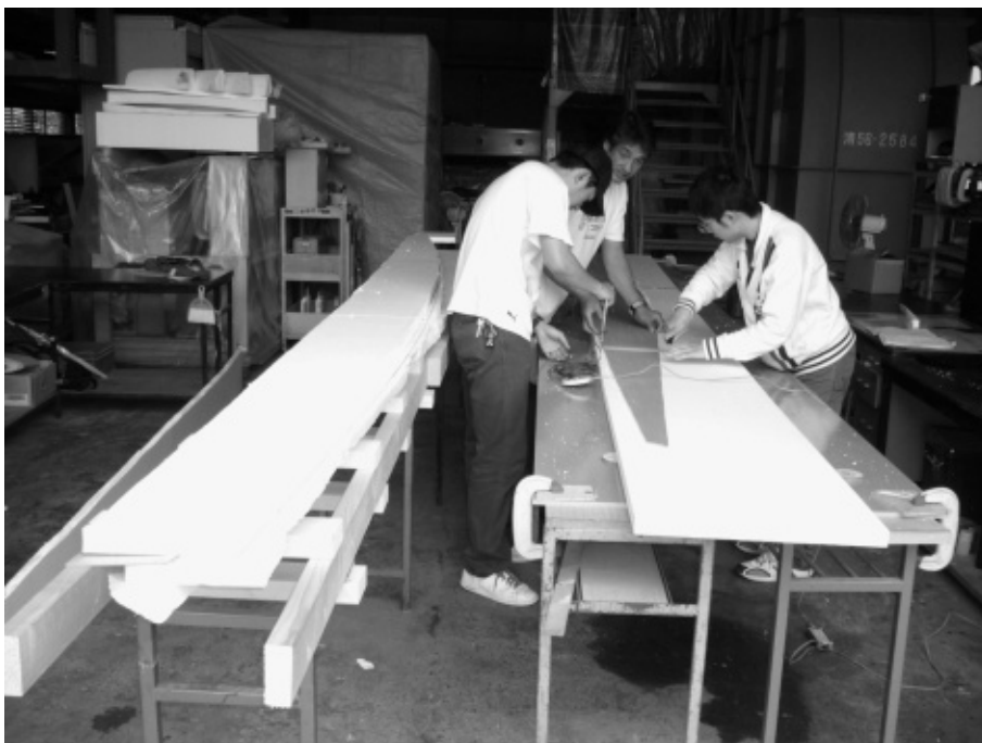
Photo 7 Rough cutting process.
