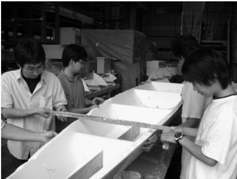
Photo 14 Free Board cutting process. Using two side gauges, hot wire cutter can easily cut both deck lines and formed bulkhead.
