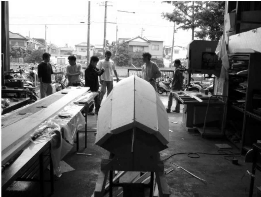
Photo 11 View from stern. Four panels are set in the ship hull form.
